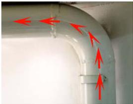
Terminator models use a large 1.50" diameter tubing with smooth radius style elbows in a 360 degree design inside the spray chamber for a non restrictive water flow
