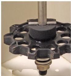
Gear driven turntable with spring loaded safety clutch engages in turntable that guarantees consistent turntable rotation within the spraychamber for a complete cleaning job.
