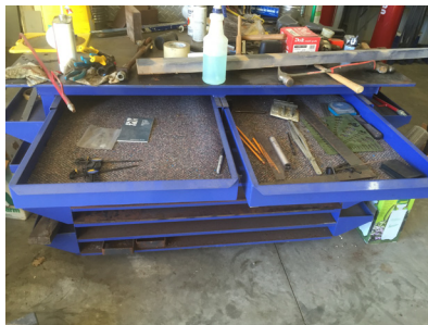
Custom 6 sided steel work bench 42" x 42" x 36" tall 3/16" plated top
