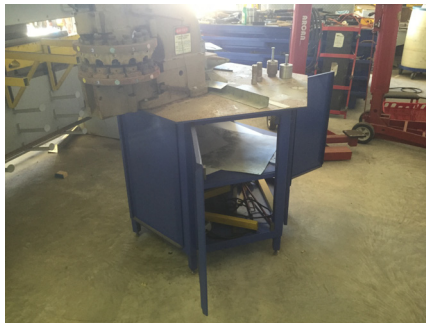
Custom 6 sided steel work bench 42" x 42" x 36" tall 3/16" plated top
