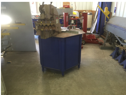
Custom 6 sided steel work bench 42" x 42" x 36" tall 3/16" plated top
