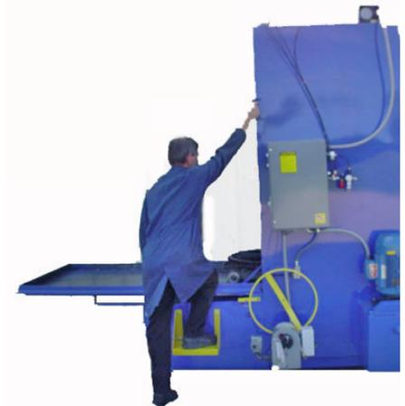
No need to reach into the spray chamber to pull out the work piece. Our handy rollout wheel feature allows you to simply turn the wheel, driving the work piece out of the spray chamber. It is safe, convenient, and fast
