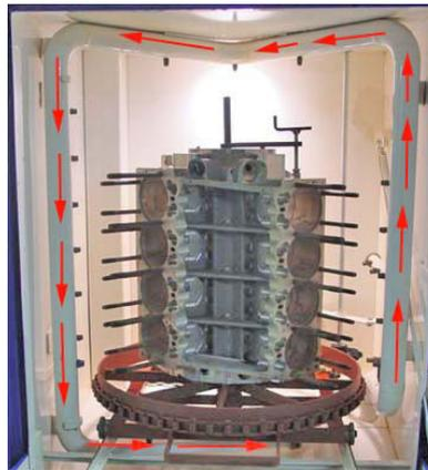
All Axe Equipment water manifolds incorporate Full 360 degree manifold constructed from 2" tubing and designed with radius elbows for high performance water flow. The SW-3660 uses a powerful 15 hp pump pushing 225 gpm at 80 psi through 27 perfectly placed nozzles for fast and efficient cleaning. (Model SW-2832 shown)
