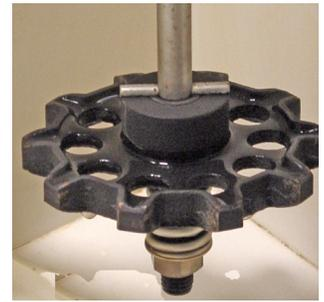
Gear driven turntable with spring loaded safety clutch guarantees consistent turntable rotation within the spray chamber for a complete cleaning job.
