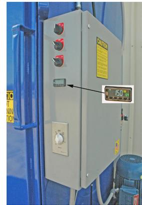
Heat is very important in the cleaning process and that is why every AXE Equipment washer is outfitted with a digital temperature controller for controlling and monitoring the heat process in the tank.
