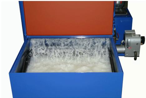
When cleaning in the spray chamber, the powerful 15 HP Pump agitates hot cleaning solutions through the 24" x 44" x 11" built in hot tank. This feature permits blocks, heads, or small parts to be hot tanked prior to spraywashing at no extra cost.
