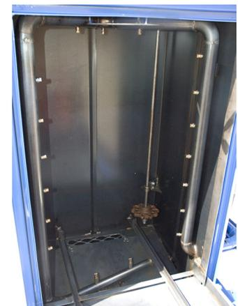
A well designed spray manifold is a key component for good cleaning. The Blue Max series uses large 2" diameter tubing with smooth radius style elbows in a 360 degree design inside the spray chamber for a non restrictive flow. Couple this design with its 5 hp pump and you get 80 gallons of hot water every minute over the parts inside with 50 psi of pressure for quickly sheering away grease and grime.
