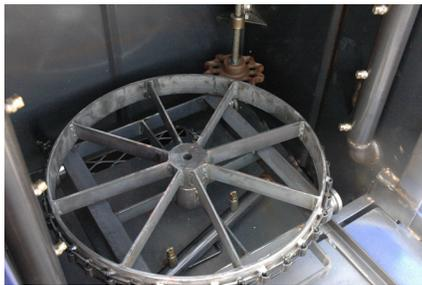
Gear driven turntable with spring loaded safety clutch guarantees consistent turntable rotation within the spray chamber for a complete cleaning job.
