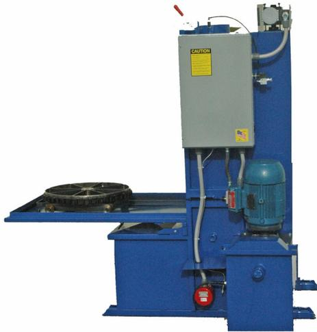
Lay down door and rollout turntable makes for easy loading and unloading. Lay down door keeps the shop floor drier and cleaner.
